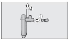
■ Remove the two rubber stoppers (①) and manually clean these and the jets thoroughly. If required, remove the air intake tube (②). Any blockages can be dislodged by kneading or "blowing through" the tube.
